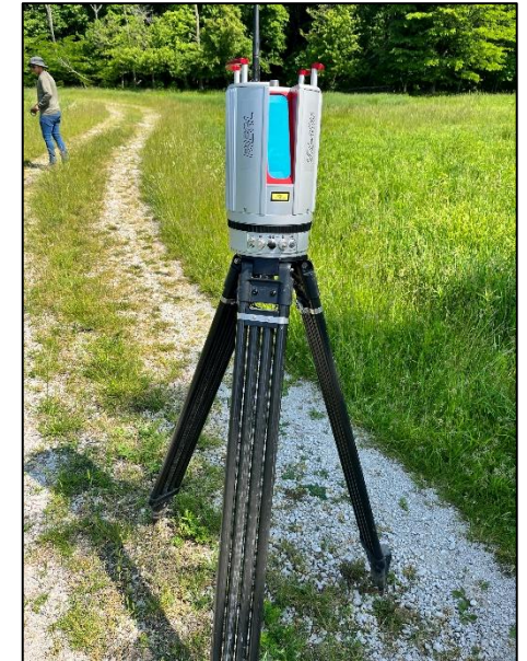
LiDAR scans to reveal channel bank migration
