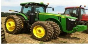
Decreasing inflation pressure while maintaining axle loads reduces soil contact pressures
