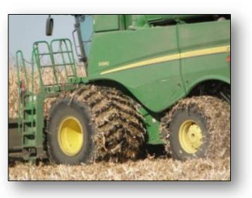
Cyclic Load per T&RA standards - Bias Flotation: + 100%: + 5 psi - Radials: + 70%: + 25% psi - IF/CFO: + 55%: + 0 psi
